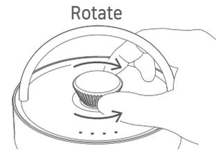
When light is on, rotate dial clockwise to increase brightness. Rotate dial counterclockwise to decrease brightness.
