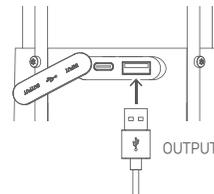
Open the rubber cover on the back of the main unit and connect the USB cable to the charging port to initiate charging. When charging, charging indicator will light up.
