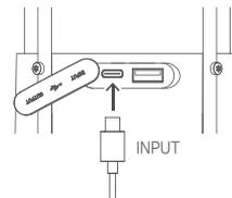
Open rubber cover on the back and connect USB-C type cable to charge lantern. When charging, battery indicator will flicker. If indicator does not blink and stays lit, it indicates charging is complete.
